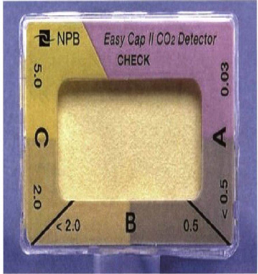
Figure 1-4. Positive detection of CO 2 turns the indicator yellow, indicating tracheal placement of the endotracheal tube.
